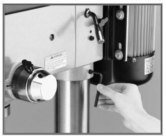
Figure 16. Tighten setscrews to secure headstock.
